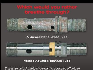
This is an actual photo showing the corrosive effects of sea water on regulator breathing inlet tubes following a six-month continuous exposure "soak" test. A competitor's conventional brass tube (top) simply cannot compete with the Atomic Titanium breathing tube (bottom) which shows no corrosion. Even an Atomic Brass breathing tube is Zirconium-plated and would not experience the level of corrosion of the competition.
