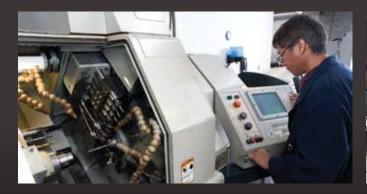
This Swiss-style CNC machine is well known for its high-precision ability in making small parts. such as those used in watchmaking.
