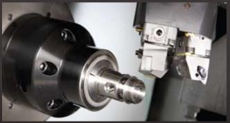
Atomica CNC machines are selected to be the best at the functions they perform. A Titanium first stage body is machined with 23 precision operations in one session.
