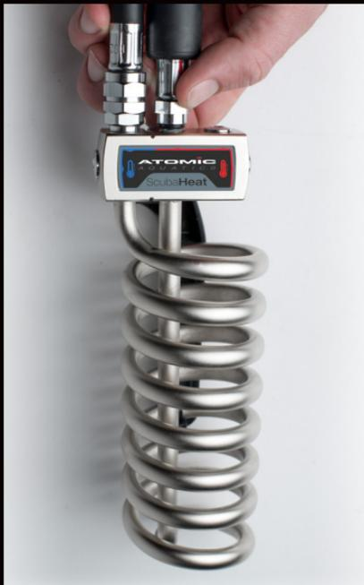
2. Next, select one of the LP ports on the warm side of the manifold indicated by the red temperature icon and install the 3/8-24 male end of your second stage hose. The top port is recommended so the regulator hose can pass over your right shoulder. Snug all connections with a wrench and pressurize to check for leaks. Do not use the end port on the cold side of the manifold.
