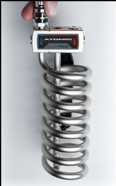
1. The first step is to install the short 11" hose included with ScubaHeat. Screw the large end fitting of the hose the into the 9/16-18 threaded fitting on top of the ScubaHeat manifold block. This is the cold side of the manifold, indicated by the blue temperature icon on the decal.
