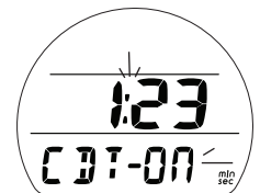
Fig. 89 - CDT STATUS (On, running)
