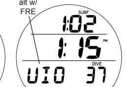
Fig. 105 - FREE VIOLATION (after 1 min on surface)
