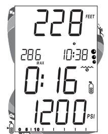
Fig. 70 - User Set Gauge Mode (Air Time Remaining)
