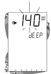
Fig. 21 - Set Max Depth Alarm
