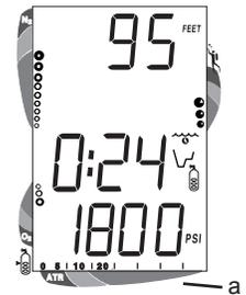
Fig. 48 - Air Time Remaining Bar Graph
