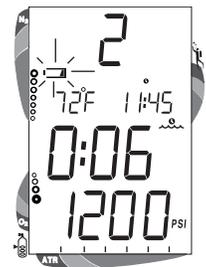
Fig. 9 - Low Battery Condition
