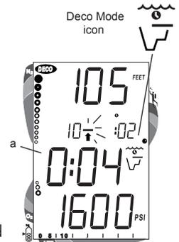
Fig. 55 - Entry into Deco Mode
