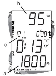
Fig. 6 - Cylinder Pressure and Depth Displays
