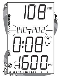
Fig. 67 - PO<sub>2</sub> Alarm
