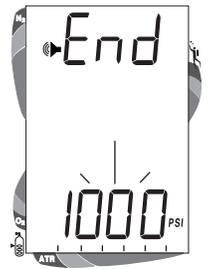
Fig. 35 - Set End Pressure Alarm
