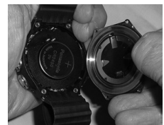
Fig. 166B - LIFTING BATTERY COVER OFF
