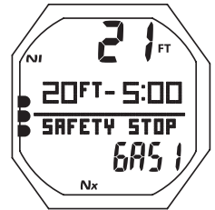
Fig. 74 - SAFETY STOP MAIN (Stop Depth/Time set)
