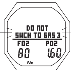
Fig. 103 - GAS SWITCH ALARM
