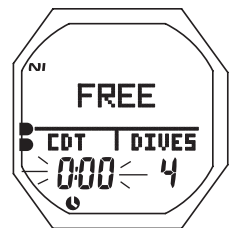
Fig. 129 - SURFACE MAIN (during CDT alarm)
