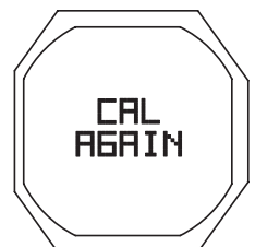
Fig. 148A - CAL FAILED
